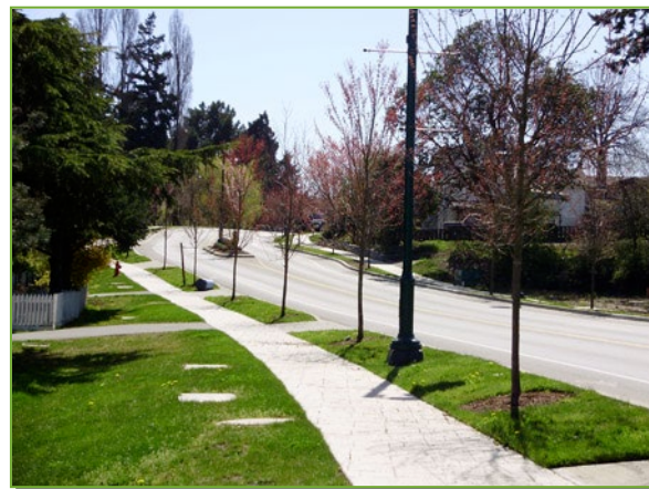
Medians, landscaping, sidewalks and bikes lanes slow down traffic, increase safety for pedestrians and cyclists, and beautify the street.
